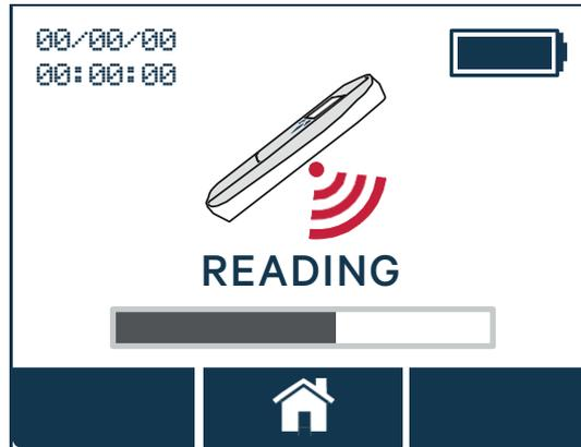
If a microchip is detected the scanner will emit a beep sound and the ID number will appear on the screen. The scanner allows the ID number to display in the ISO 15-digit format. When a microchip is detected, the following information will be displayed: 15-digit ID, manufacturer or country code (if applicable), and below that, the type of RFID Microchip detected. If no microchip is found within 60 seconds “Tag not found” will appear on the scanner’s screen:
