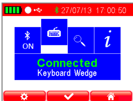
Fig. 7 Reader is connected in Keyboard Wedge profile
