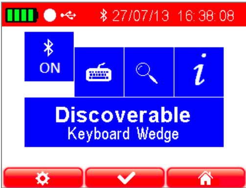
Fig 3. The Bluetooth menu. On opening this menu, the Bluetooth on/off option is active.
