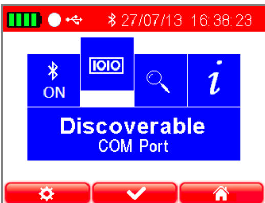
Fig 4. The device is now “Discoverable” by another Bluetooth device. Here the “COM” profile has been selected (1010 symbol).
