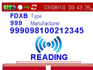
OMNI MAX will give an audible sound and you will hear a “beep” when the scanner successfully detects a microchip.
