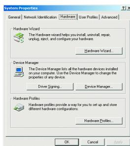
6. Select in the Hardware tab the Device Manager to discover the Communication port assigned.
