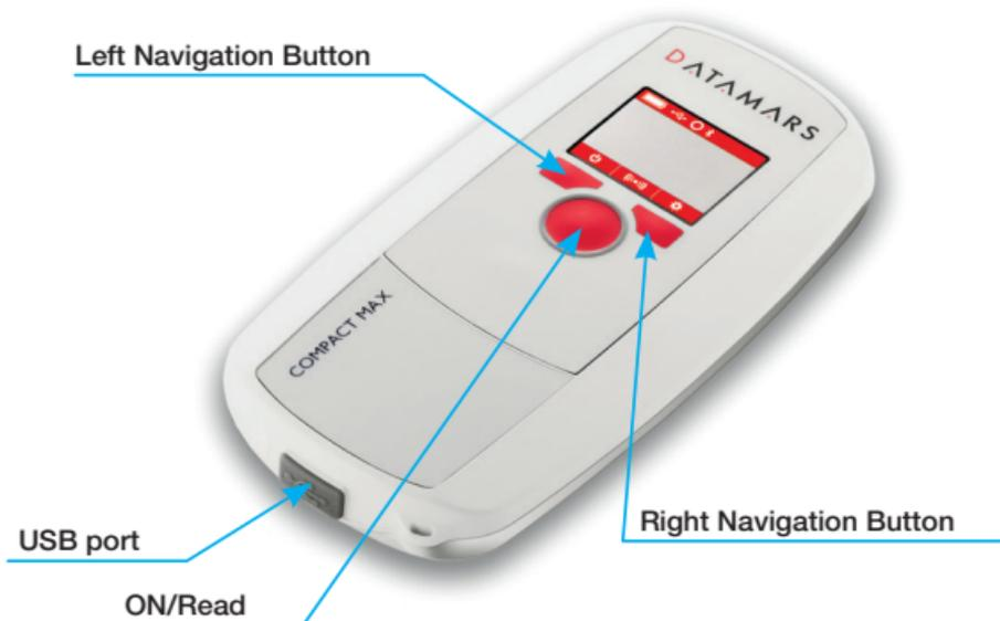
To conveniently interface COMPACT MAX to your computer, to check for newer versions of the COMPACT MAX firmware or to modify the default settings, we recommend using S-ID companion software, freely downloadable from [www.pet.datamars.com](http://www.pet.datamars.com)
